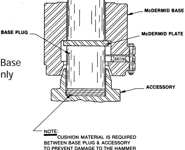
We do not recommend the use of McDermid bases for any type of pile other than wood. But on occasion, contractors have found themselves in a position where they have had to adapt a McDermid base to standard Driving Heads or Pipe Caps. The above shows the arrangement necessary to accomplish this.
