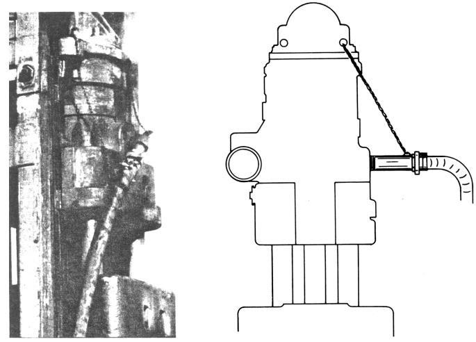
The length of the Nipple from the Inlet must be kept to a minimum. A long Nipple, as shown in the drawing, even though supported by chain or wire rope, will cause damaging leverage and vibration. Extensions to the side, like the arrangement in the picture, allow for good support of the Piping and Hose.
