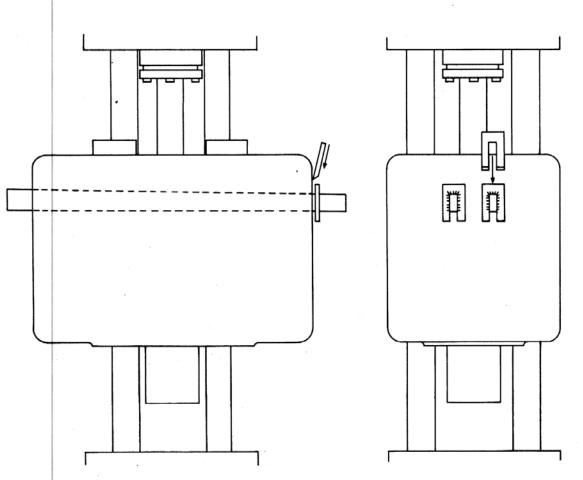
When some hammers get enough mileage on them to warrant retirement and under certain driving conditions, the contractor may have trouble keeping the ram keys tight. Usually under these circumstances, the contractor will weld the keys to the ram and worry about the consequences later. The drawing above shows a better way of keeping the keys tight and allows for quick and easy retightening during the job.
