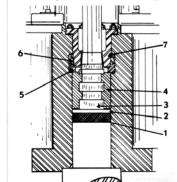
four Dowel Pins, align the Ram Retainer Split Ring (7) around the Piston Rod and insert into Segmental Pressure Ring as shown. Securely fasten all hold-down nuts.
