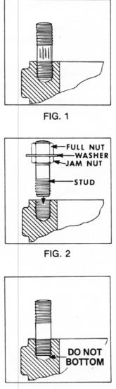
All Vulcan studs have an unthreaded portion between the two threaded ends. DO NOT install studs using a pipe wrench on the unthreaded portion of the stud. Aside from possible damage to the threads, the marks or notches (Fig. 1) made by the pipe wrench create stress riser points in the stud.
