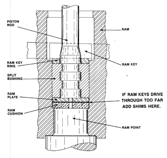
After a Hammer has a lot of "mileage" the parts that hold the Piston Rod to the Ram wear a little. This will necessitate some adjustment to insure proper tension of the Ram Keys. If this condition exists in your Hammer and the Ram Keys have a tendency to drive through too far, add Shims between the Ram Cushion and the Ram Plate.
