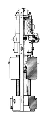
The Differential system requires 1/3 less air or steam as compared to a similar size Double Acting Hammer.
